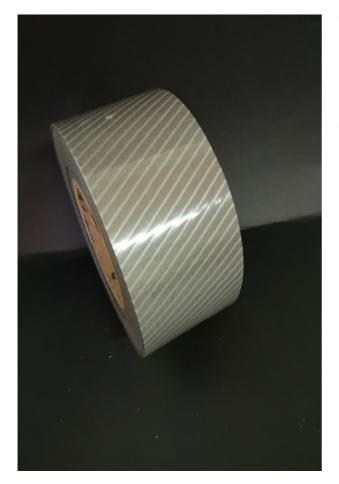
The product basically consists of segmented metallised microspheres, partially incorporated in a removable polyester (front layer) and permanently bonded to a thermoadhesive (backing layer). The thermoadhesive polyester base provide excellent adhesion to the most common type of fabric,
