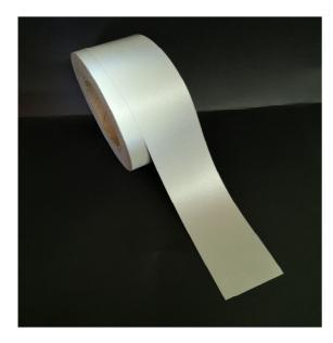
The product basically consists of a fabric coated with metallised microspheres having known reflective index and extremely high refraction power, by means of a polyurethane binder with high flexibility and resistance to mechanical and chemical-physical stresses.
