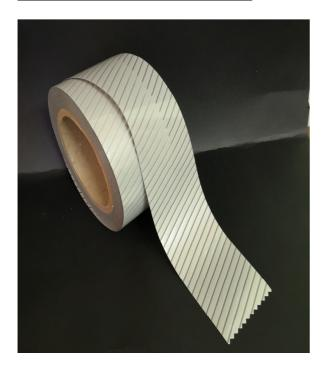
The product basically consists of segmented metallised microspheres, partially incorporated in a removable polyester (front layer) and permanently bonded to a thermoadhesive (backing layer). The thermoadhesive polyester base provide excellent adhesion to the most common type of fabric,
