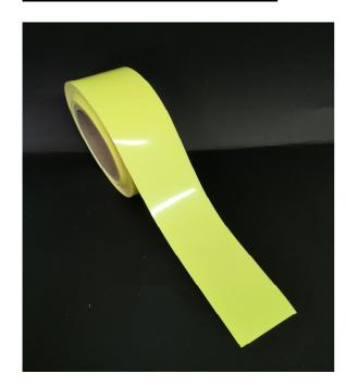
The product basically consists of metallised microspheres having known reflective index and extremely high refraction power, partially incorporated in a removable polyester (front layer) and permanently bonded to a thermoadhesive (backing layer). The thermoadhesive polyester base provide excellent adhesion to the most common type of fabric, with high flexibility characteristics for a higher resistance to the finished product.
