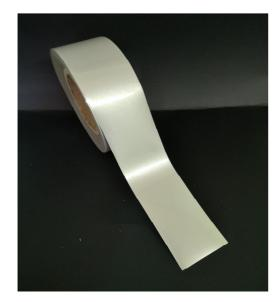
The product basically consists of metallised microspheres having known reflective index, partially incorporated in a removable polyester (front layer) and permanently bonded to a **FLAME RETARDANT** thermoadhesive (backing layer). The FR thermoadhesive polyester base provide excellent adhesion to the most common type of fabric, with high flexibility characteristics for a higher resistance to the finished garment.
